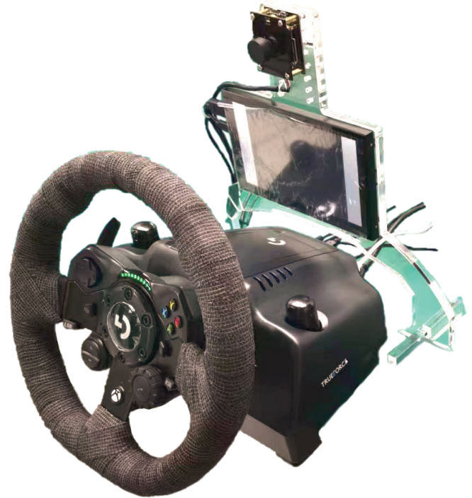
Complete demo for DMS. Parts you can see are: Steering wheel [has the cap sense fiber], LCD, Camera and IR LED
